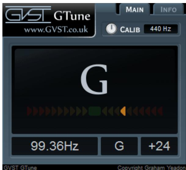
The GUI has four parts. From top to bottom these are the reference frequency control, the main display, the coarse-tune "LED" indicators and the frequency readout.
