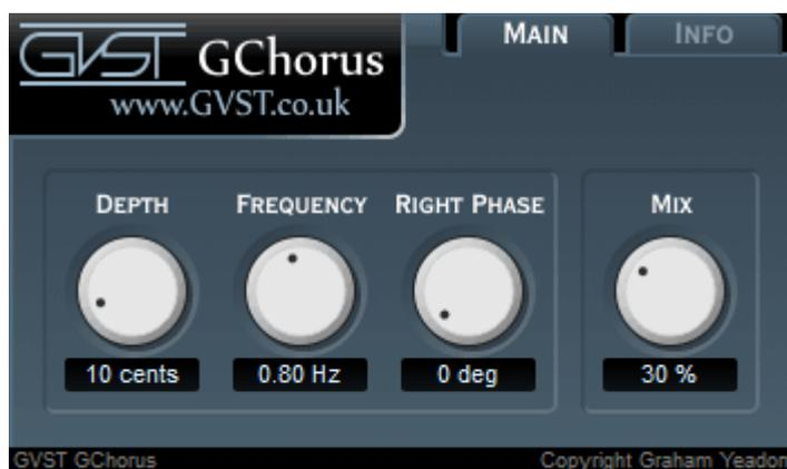
The GUI features four knobs which control all of the plug-in's parameters. Each features a label above, and an editable readout below.
