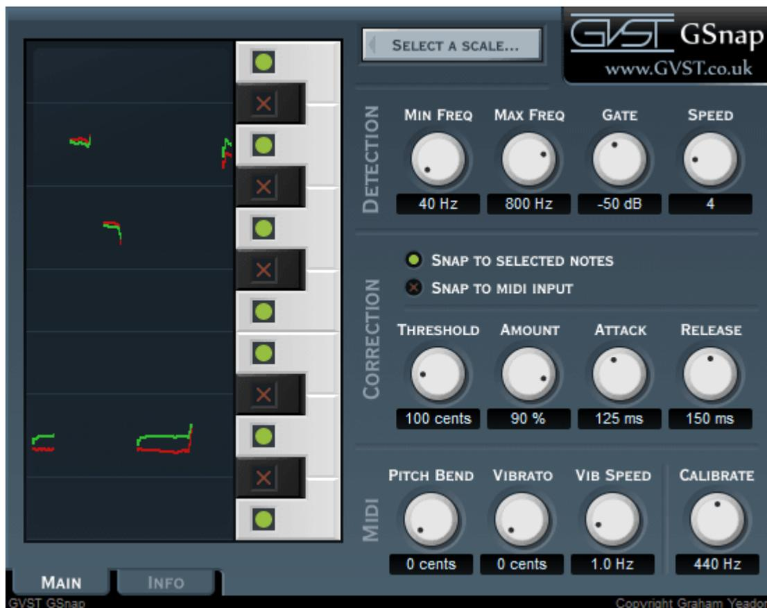
The GUI features a set of 12 knobs which control all of the plug-in's parameters. Each has its function clearly labelled above, and features a user-editable readout below. Additionally, twelve "switches" next to the pitch data view correspond to the twelve semitones of a full octave in the Western chromatic scale, and are used to supplement the "fixed" mode of GSnap. Two further switches allow the user to select between "fixed" or "midi" modes, explained below.
