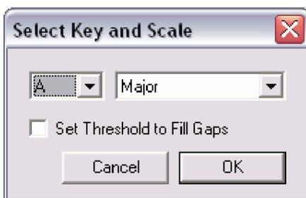
A drop-down menu allows you to select the "root" of the scale, and another the "mode". Checking the "Set Threshold..." option will automatically adjust the Threshold parameter so that the chosen scale is enforced.
