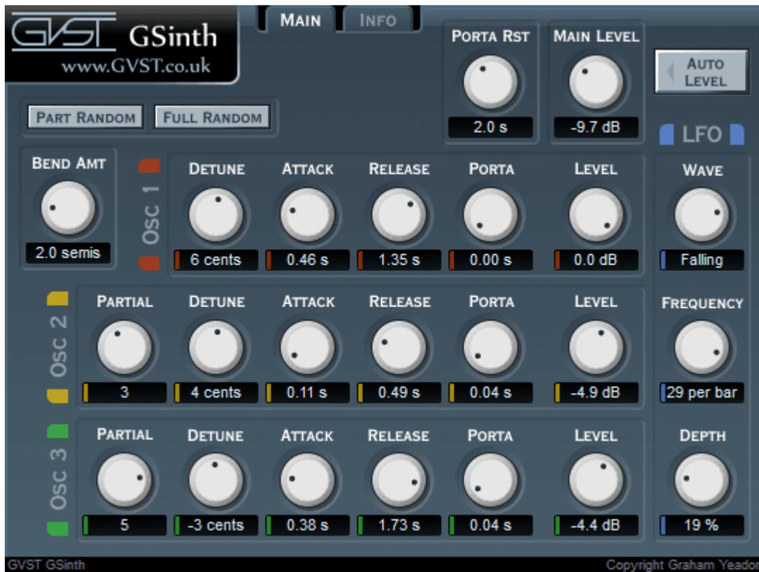
Each knob is laid out the same way for consistent and easy reference. Above each one, its function is labelled. Below each one is a numerical readout of the value assigned. There are also two buttons to aid configuration, "Random" and "AutoLevel".
