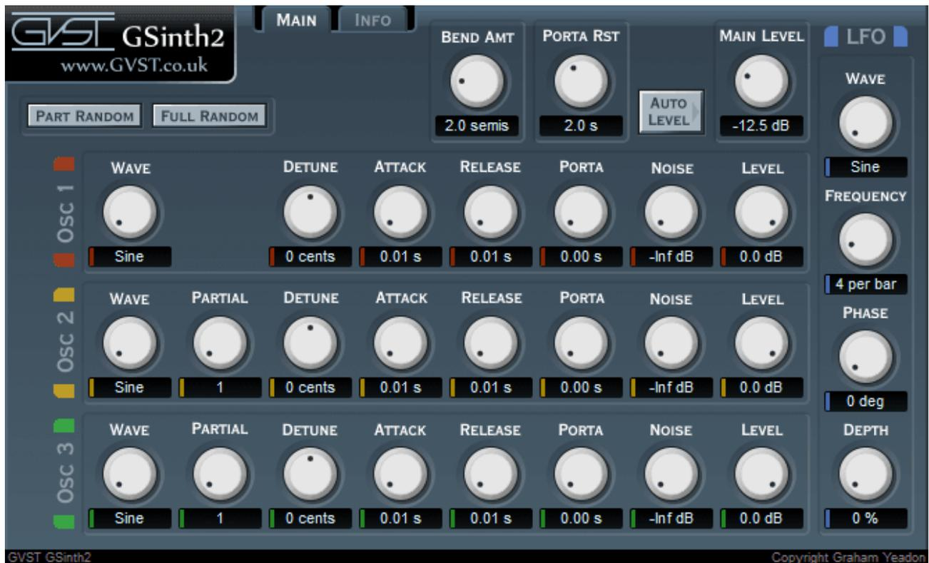
Each knob is laid out the same way for consistent and easy reference. Above each one, its function is labelled. Below each one is a numerical readout of the value assigned. There are also two buttons to aid configuration, "Random" and "AutoLevel".
