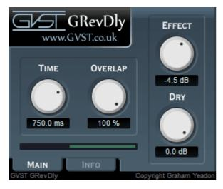
Four knobs control GRevDly's parameters. Each is clearly labelled above, with a user-editable readout below. Embedded into the GUI is an illustration of the signal path.
