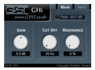
The three knobs are presented the same way for consistent and easy identification. Above the knob, its function is labelled. Below the knob, a numerical readout reflects the user adjustments or allows the user to manually specify values. One additional mini-window at the bottom of the GUI shows the peak level of the outgoing signal, in decibels.
