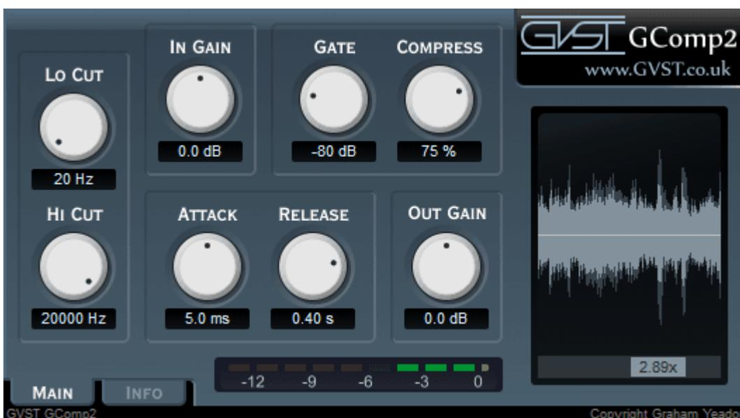
The GUI features a set of 8 knobs which control all of the plug-in's parameters. Each is clearly labelled above, with a user-editable readout below.
