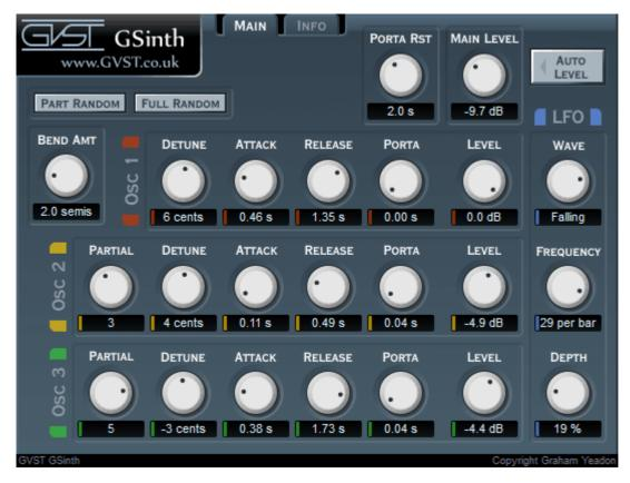
Each knob is laid out the same way for consistent and easy reference. Above each one, its function is labelled. Below each one is a numerical readout of the value assigned. There are also two buttons to aid configuration, "Random" and "AutoLevel".
